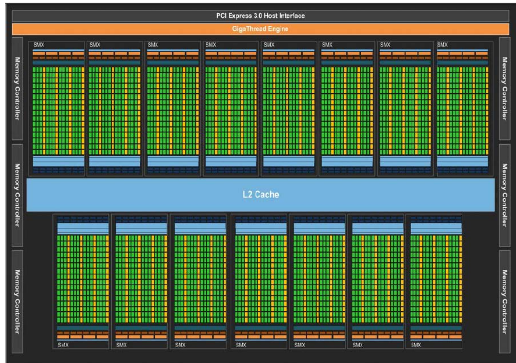
Figure 3.19 NVIDIA Kepler GK110 architecture
